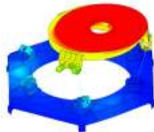
Mode 2 @27 Hz Hexapod mode with rigid body translation of the M4AM along X-axis.
