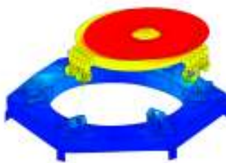
Mode 1 @27 Hz Hexapod mode with rigid body translation of the M4AM along Y-axis.
