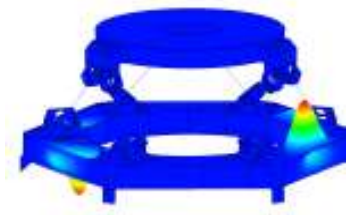
Mode 3 @40 Hz M4MS local mode ; no influence on the M4AM (modes 4 to 9 are similar to mode 3)
