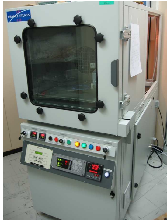
Figure 5: High vacuum bakeout used during the cleaning of the laser source
