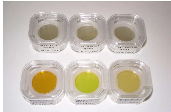
Figure 3: ZnSe mirrors used in the OPO stages manufactured by CILAS Aubagne (France)
