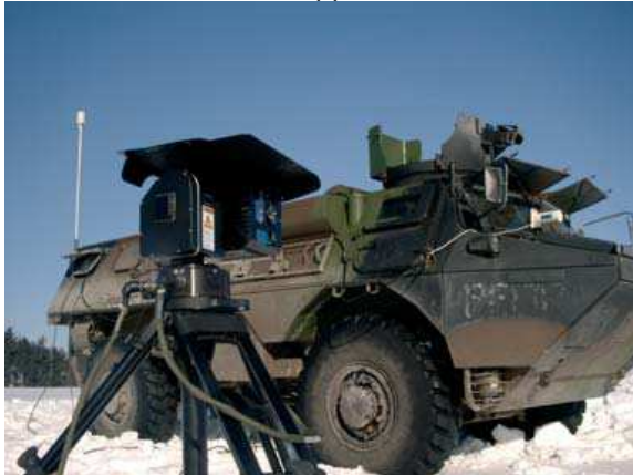
Figure 2: SLD500 used as a remote display unit for sniper detection from a VAB (CILAS product)
